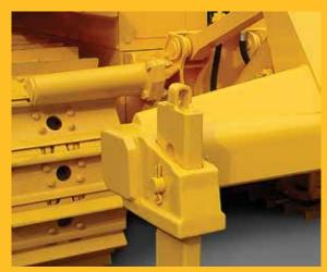
Dressta landfill dozers are equipped with track shoes with center clean-out holes. These reduce the risk of materials jamming the track componentry between the sprocket and track chain bushings which cause accelerated wear and tear.
