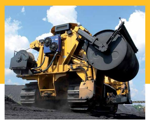
Dressta machines adapted for stockpile applications have their weight spread across the sturdy undercarriage for superior balance and stability. With the compaction equipment installed, these dozers can operate on lengthwise slopes of 25° and crosswise slopes of 20°.
