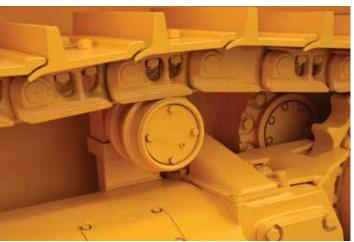
Working loads from the blade and rear mounted attachments are evenly distributed through the frame and undercarriage.
